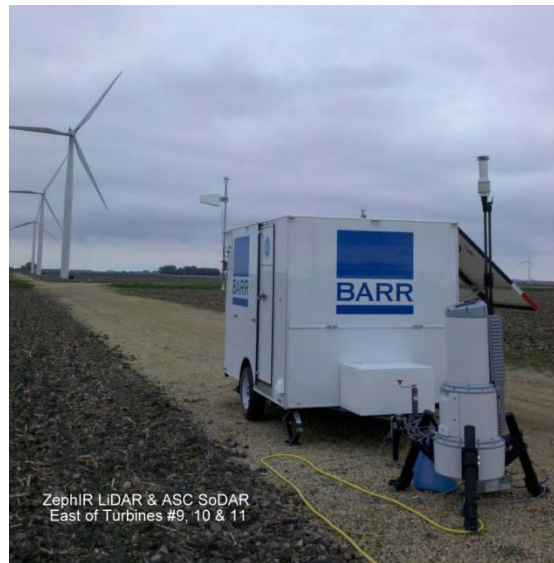
Fig. 12. Wind Farm in the Mower county area (top) and LiDAR in operation in the wake of a wind turbine (bottom).
