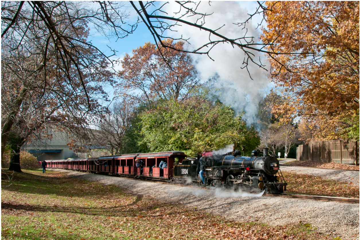
BELOW: The two steam locomotives of the Milwaukee County Zoo burning torrefied biomass fuel during test runs in November 2017.
