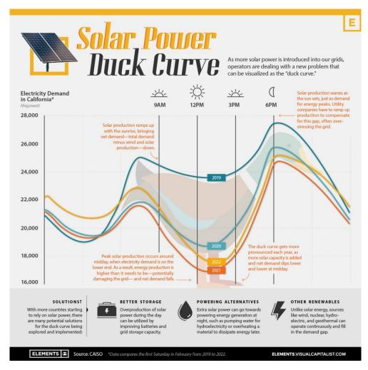
The ramp needed in California in 2022 for the midday low to the peak demand in the evening was approximately 13000 MW within three hours. This is an example of why 24/7 dispatchable generation from advanced nuclear and or a new gas plant with carbon capture could be beneficial to Xcel Energy and its customers, as well as to Pueblo.
